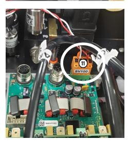
**16.** Install the 2 CAN cables ② on the mixer module. Use your fingers to tighten these connections. Do not use tools. Tools can damage these connectors. Do not cross-thread the CAN cable connectors. If these connections are cross-threaded, they are not easy to remove.
