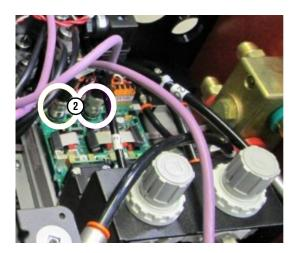
**4.** Remove the manifold-side panel to get access to the mixer module (229703). This manifold-side panel has the 24 V power supply (229640) and control PCB (141375) attached. Refer to Gas connect console panels on page 100.
