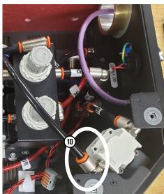
15. Connect the SV100 (1) connector to the mixer module.
