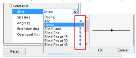
Pinned lead styles are saved with the ProNest machine, so that machine-specific lead styles will always be readily available.
