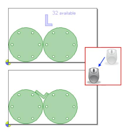
When dragging a part on the nest, the part will bump up against existing parts or plate edges and then rotate to fit. You can glide the part along edges of neighboring parts to get the best result. This makes it easy to fit parts into empty spaces on the nest, without the need to manually rotate the part to just to right angle.
