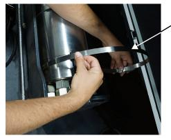
5. Put the ends of the guard straps into the bolt drives.
