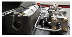
4. Put the guard straps inside the guard and around the attenuator.
