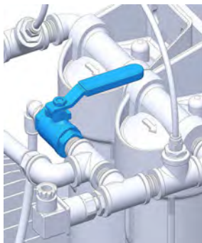
Water valve in closed position
