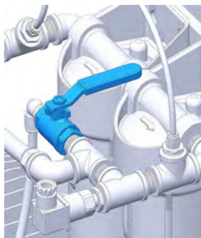
Water valve in closed position
