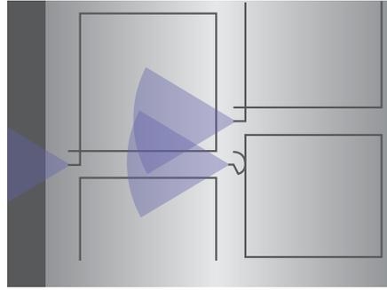
Leads are appropriately placed and use a moving pierce. This ensures that the direction of the molten splatter is a predictable "splash zone," directed off the plate or towards parts already cut, with easily removable slag.
