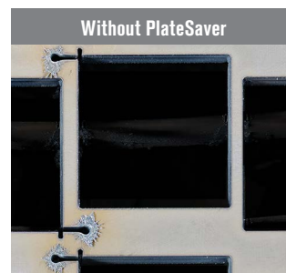
Traditional leads require more space between parts.
