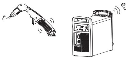
3. Pull the torch trigger again to fire a plasma arc.
