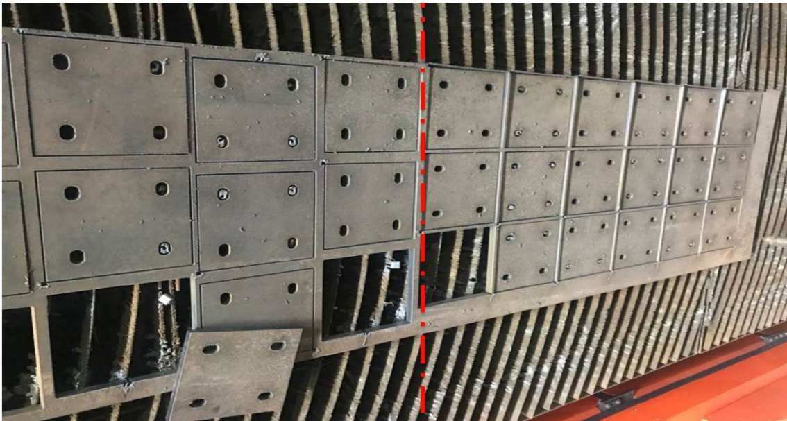
Figure 2 – Sample cut showing results from nesting with standard leads (left of the dashed line) compared to Plate Saver leads (right of the dashed line). Skeleton with Plate Saver leads highlights reduced scrap around parts
