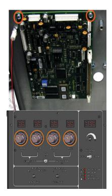
Remove the screws using a Phillips screwdriver. Remove the switch hardware by hand.
