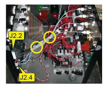
Remove the screws using a Phillips screwdriver. Unclip and remove all cables.
