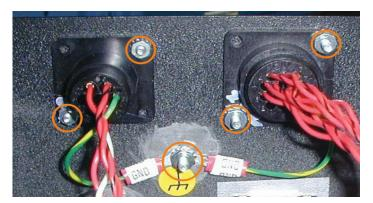
Remove the screws using a Phillips screwdriver. Pull to remove wires from their connectors.
