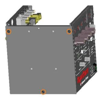
Remove the screws using a Phillips screwdriver. Pull to remove cables and wires from their connectors.
