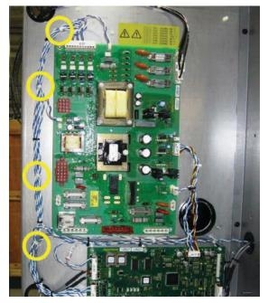
Cut all the cable ties and remove the wires from their connectors.
