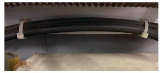
Remove the nuts using a 9/16 inch socket. Cut all the cable ties.
