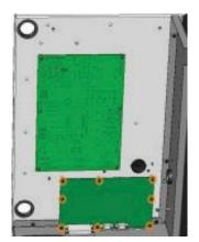
Use a Phillips screwdriver and the T25 TORX driver to remove the screws and bolts from the control board and from all four corners of the power distribution board.
