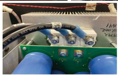
Remove the wires from the plastic cable holders by pulling to remove the wires from their connectors. Remove the screws with a 7/16 inch socket. Cut all the cable ties from wire to tab.
