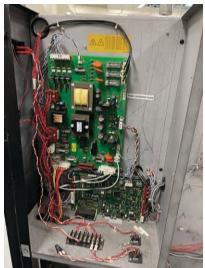
Cut all the cable ties and unplug the wire terminal.
