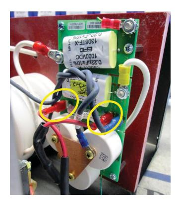
**Note**: There is no need to remove the wires. You can optionally recycle them into the mixed metal recycling stream.
