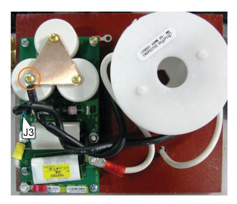
Remove the nuts using a 1/4 inch socket and a 7/16 inch socket.
