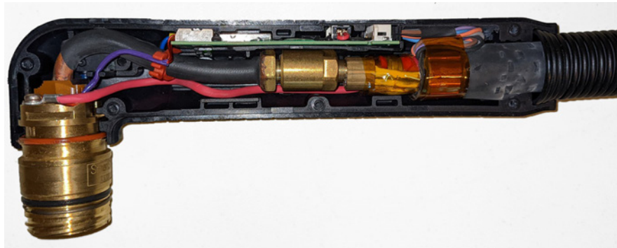
Figure 19 – 90° robotic torch components in correct positions
