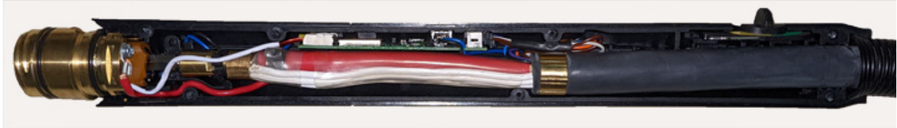
Figure 12 – Full-length machine torch components in correct positions
