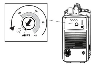
2. With the amperage knob in the gas test position, pull up on the pressure regulator knob on top of the system to unlock it.
