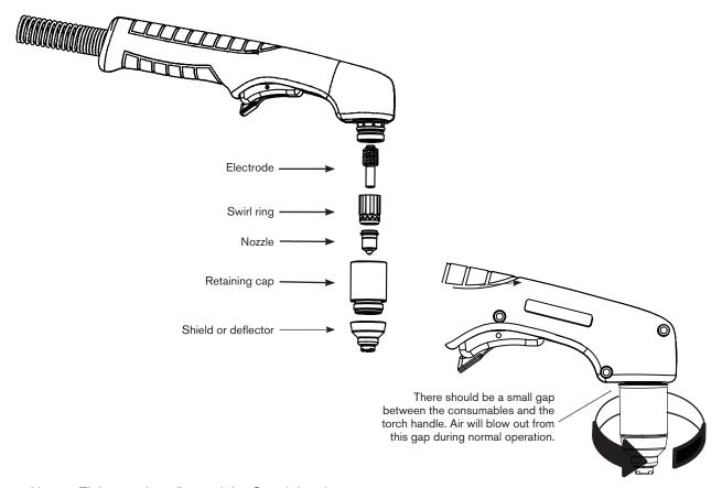
Note: Tighten only to finger-tight. Overtightening
