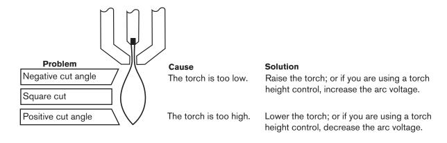
Notes: The squarest cut angle will be on the <u>right</u> side with respect to the forward motion of the torch. The left side will always have some degree of bevel.
