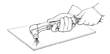
3. Maintain an approximate 45° angle to the workpiece as you feed into the gouge.
