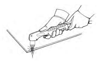
3. Drag the nozzle lightly across the workpiece to proceed with the cut. Maintain a steady, even pace.
