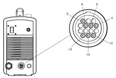
Refer to the following table when connecting the Powermax45 to a torch height controller or CNC with a machine interface cable.
