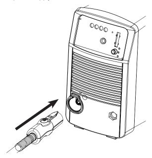
To remove the torch, press the red button on the connector and pull the connector out of the receptacle.
