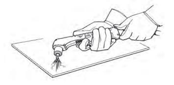
3. Hold the torch in place while continuing to press the trigger. When sparks exit from the bottom of the workpiece, the arc has pierced the material.
