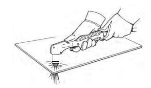
4. When the pierce is complete, drag the nozzle lightly along the workpiece to proceed with the cut.
