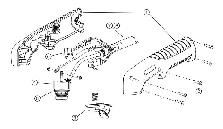
The entire hand torch and lead assembly can be replaced, or individual component parts can be replaced. Part numbers starting with 088 indicate complete torch and lead assemblies.
