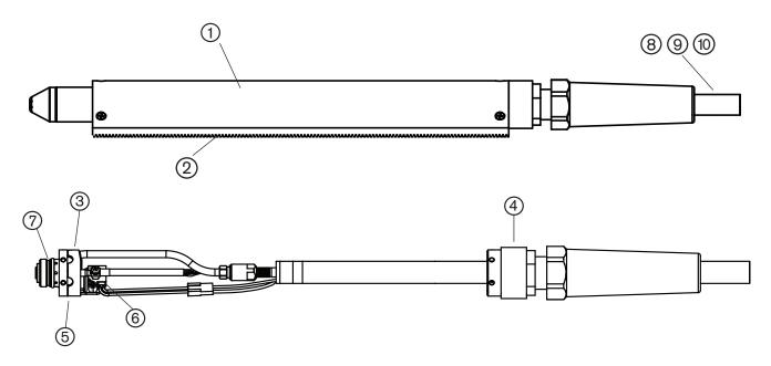
The entire machine torch and lead assembly can be replaced, or individual component parts can be replaced. Part numbers starting with 088 indicate complete torch and lead assemblies.
