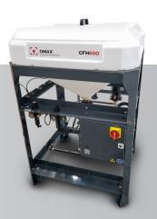
The innovative Continuous Feed Hopper improves your production times with automatic garnet delivery to the abrasive waterjet nozzle. Utilizing pneumatic pressure to transport garnet from the large capacity 600 lb (272 kg) hopper pot to the cutting head hopper, the Continuous Feed Hopper helps to eliminate unplanned downtime with the ability to fill the hopper while in use.
