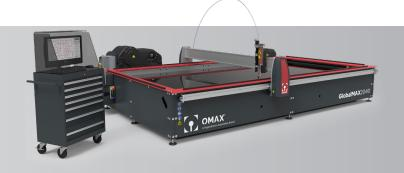
Essential, easy to use and powerful, GlobalMAX® is ideal for the facility looking to add basic waterjet cutting capabilities. The robust and straightforward design delivers dependable performance and easy serviceability to provide maximum uptime. The GlobalMAX JetMachining Center® was developed, tested, and built in keeping with the OMAX philosophy of performance, reliability, and ease of use. The GlobalMAX product line is manufactured and assembled at the OMAX facility in Kent, Washington.
