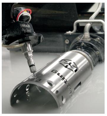
When used with the VersaJET, fishmouth intersections, saddle cuts, and countersunk holes can be cut along the circumference of pipes.
