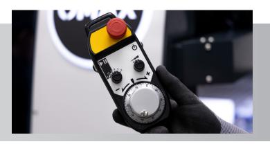
The OptiMAX® Bridge Pendant allows the waterjet operator to move the Cutting Head and the Bridge along X, Z and Y Axis, dial in the cutting head to the work piece, or perform dry runs to test drawings or material fixturing.
