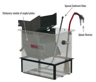
When cleaning the tank, the removable angled plate module can be lifted from the accessory unit. An operator can clean out the sediment from under the stationary angled plates by using the Special Sediment Rake.
