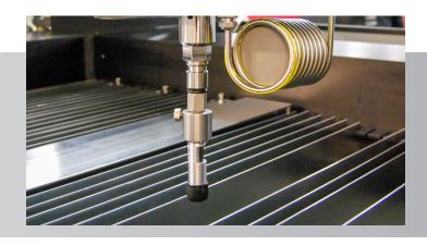
Perform simple dry runs with this laser attached to the nozzle before you cut parts on valuable stock.
